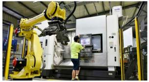
Chamberlain Group robot carrying out post-processing gauging. Many Central Coast manufacturers have embraced the latest technologies in their manufacturing process.
